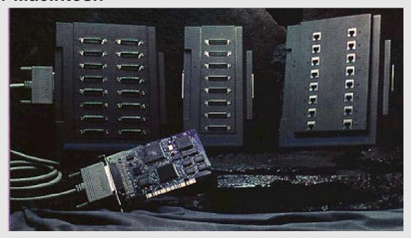
Fenris adds 8 to 64 "smart" RS-232 serial ports to your PCI Power PC Macintosh. An on-board RISC processor and half a megabyte of on-board buffering ensures minimal loading of your Macintosh while supporting serial data rates up to 115,200 baud per port. Fenris is a perfect way to support any medium to large Mac BBS, multi-line fax or mail server, or to control multiple serial hardware devices. Multiple Fenris cards may be used in a single Macintosh to provide additional ports.
