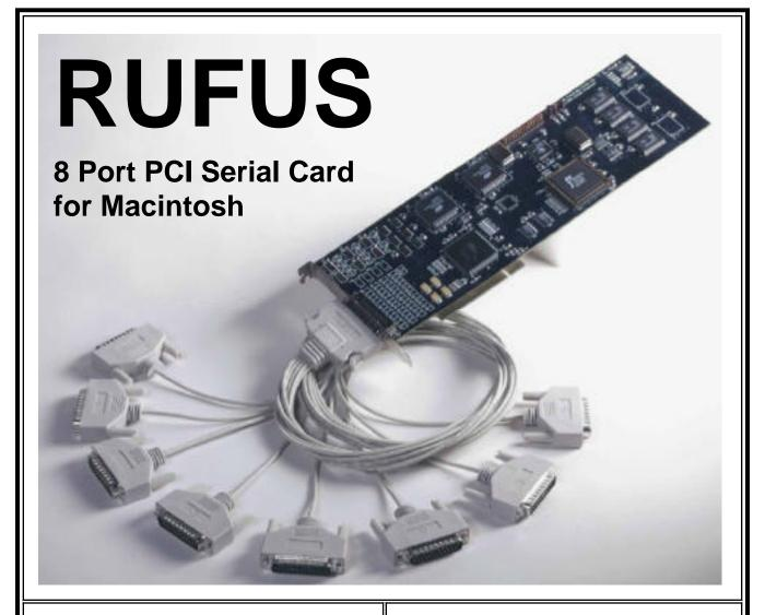
Rufus adds 8 "smart" RS-232 serial ports to your PCI Power PC Macintosh. An on-board RISC processor and half a megabyte of local buffering ensures minimal loading of your Macintosh while supporting serial data rates up to 460,800 baud per port. Rufus is a perfect way to support any small to medium sized Mac BBS, multi-line fax or mail server, or to control multiple serial hardware devices. Multiple Rufus cards may be used in a single Macintosh to provide additional ports.
